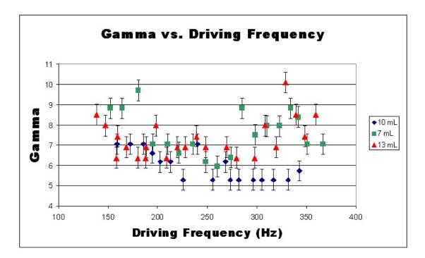
Figure 9: A chart of frequency vs.  $\Gamma$  for points at which the pattern first appears with  $\Gamma$  increasing from 0. Different colors signify different volumes, as noted on the legend at right. Error bars come from error in measuring p-p voltage as described in Section 5.
