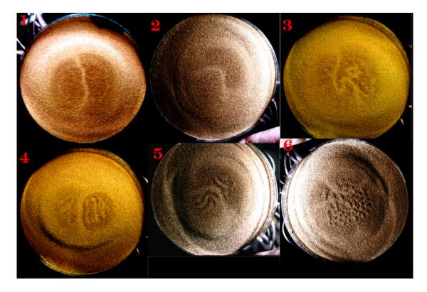
Figure 8: Different variations of the initial pattern, appearing at different  $\Gamma$  values. 1. A simple straight kink. 2. A  $\cup$ -shaped kink. 3. An S-shaped kink with a circular kink to the side. 4. A straight kink at higher  $\Gamma$ , exhibiting stripe patterns in the period-doubled regions. 5. A  $\cup$ -shaped kink with stripe patterns in the period-doubled regions. 6. Two  $\cup$ -shaped kinks with stripe patterns in the period-doubled regions.
