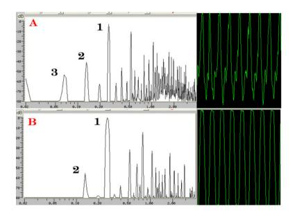
Figure 10: FFT graphics and waveform examples with driving frequency (1) and subharmonic peaks (2,3) which indicate period doubling. Figures are for A, an accelerometer under one region near the kink and B, the driving (shaft) accelerometer. The FFT diagram is on a logarithmic frequency scale, with decibels on the y-axis.
