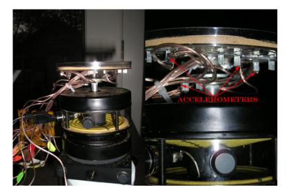
Figure 4: The shaker and Petri dish assembly attached via banana plug, showing accelerometer mounts.
