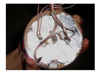
Figure 5: The bottom of the Petri dish, showing mounting of accelerometers, banana plug, and aluminum foil for static electricity dissipation.
