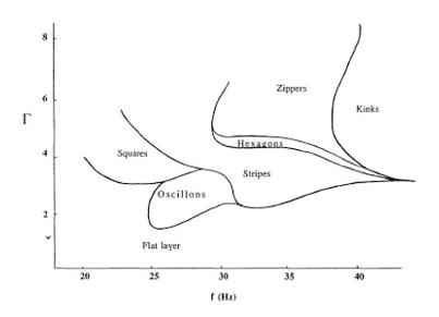
Figure 11: A phase diagram for .15-.18mm brass spheres with layer depth 20, collected with decreasing  $\Gamma$ . [3]
