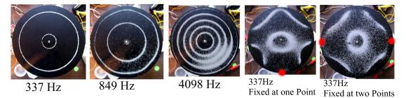
Figure 3: Pattern formation on vertically vibrated Chladni plates, thickness .092 cm, diameter 28.95 cm. Red dots indicate points held stationary during vibration.
